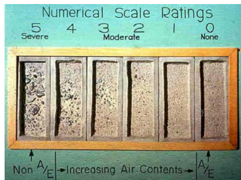
Figure 3. Illustration of the surface rating scale for visual evaluation of scaling [13]
